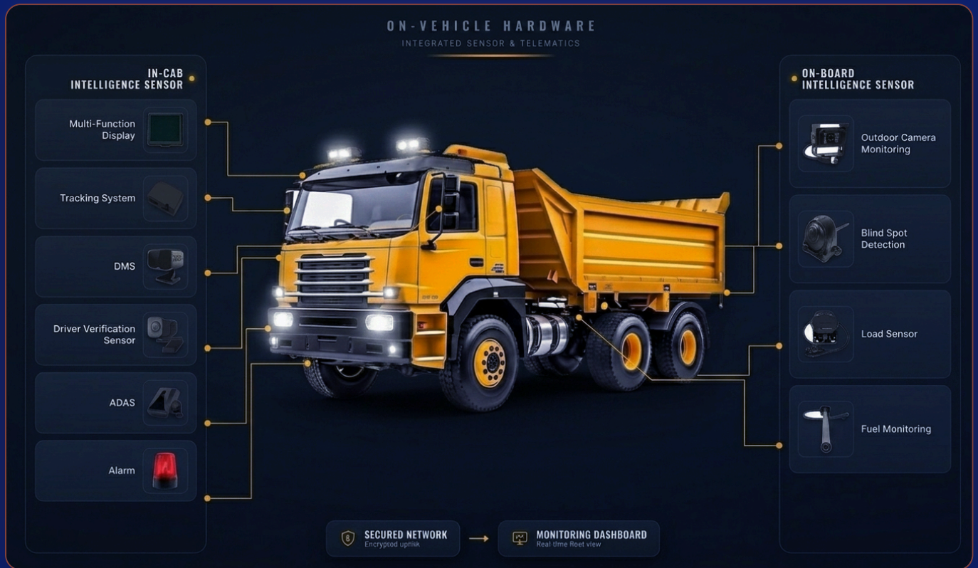
On-vehicle sensor suite — ADAS/DMS, cameras, fuel & load sensors — connected to the cloud monitoring dashboard.
